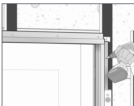
Corner profile meeting a starter profile above an opening
