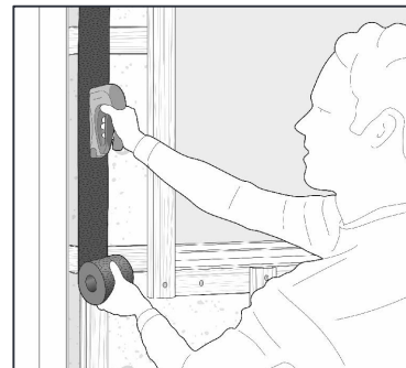
Cover all battens with EPDM strip
