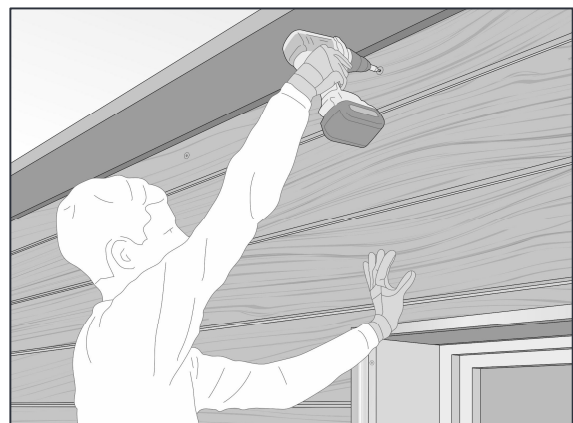
Face fixing the last row of Cedral Click using Cedral face fixings
