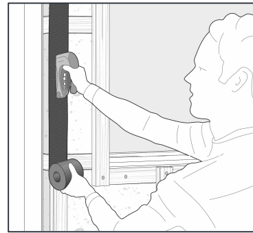
Cover all battens with EPDM strip
