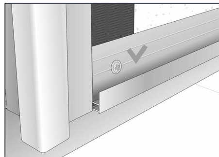
Use Cedral Click clip screw or rivet for fixing of the starter profile to support frame. Ensure the screw or rivet sits flush with the profile surface.
