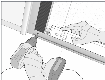
Ensure the starter profile is installed true level and next to the corner/end profiles
