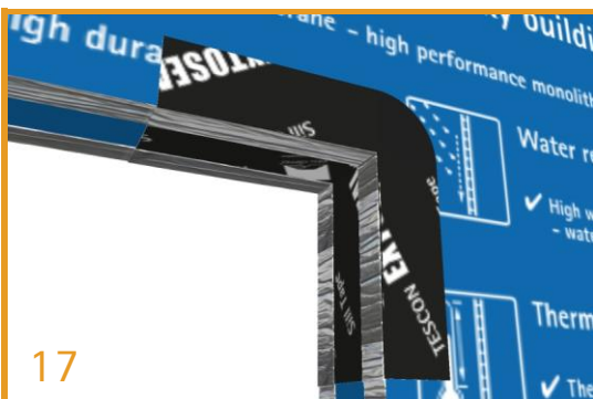
Continuous TESCON® ADHISO WS TESCON® ADHISO WS back seal should be continuous around the entire window. The front seal will be continuous on the jambs and header only.
