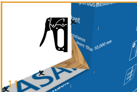
Fixing the Reveals The flaps should be fixed into the window reveal using staples at the rear edge of the window reveal spaced evenly at 150 mm centres.
