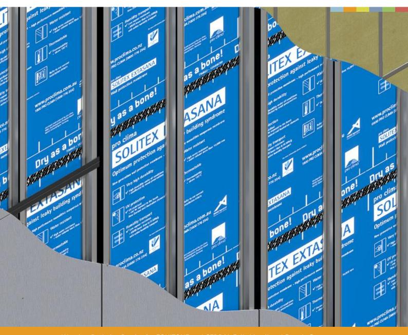
Weather Resistive Barrier for EQUITONE and CEDRAL Fully Ventilated Façade System
