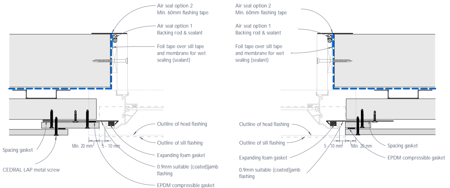
Figure 18: CEDRAL LAP typical flange window jamb junction or the like - Flush detail
