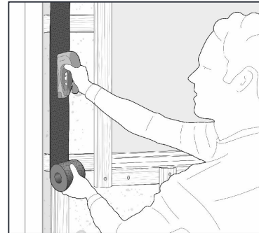
Cover all battens with EPDM strip
