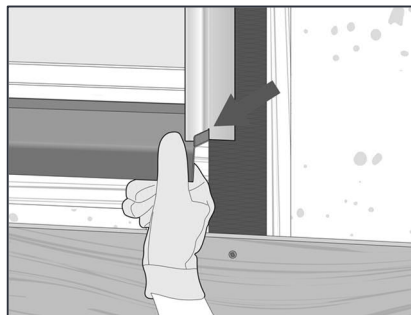
Cut the jamb profile or flashing and adequately notch it at the bottom to accommodate the window sill upstand. It is recommended that the sill flashing has a minimum 15 mm upstand at each end.
