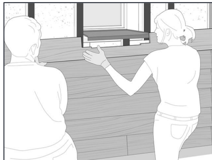
Install the trimmed plank, which now matches the window and sill. Take extra care not to break the plank where the edges have been cut out.
