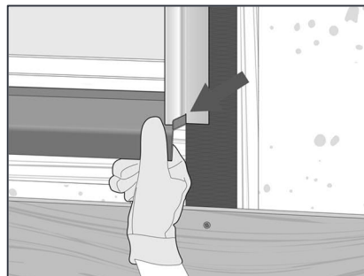
Cut the jamb profile or flashing and adequately notch it at the bottom to accommodate the window sill upstand. It is recommended that the sill flashing has a minimum 15 mm upstand at each end.
