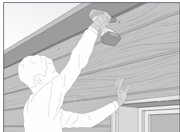
Face fixing the last row of Cedral Lap using Cedral face fixings
