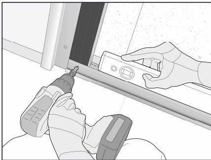
Ensure the starter profile is installed true level and next to the corner/end profiles
