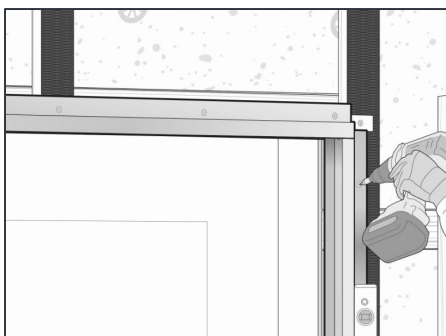
Corner profile meeting a lintel profile above an opening
