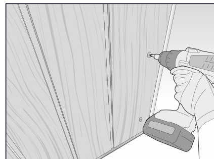
The first and last planks are face fixed using Cedral face fixings on the clipless side of the plank with adequate edge distance.
